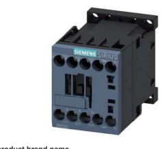
Power contactor, AC-3 7 A, 3 kW / 400 V 1 NO, 110 V AC, 50 Hz 120 V, 60 Hz, 3-pole, Size S00, screw terminal upright mounting position
