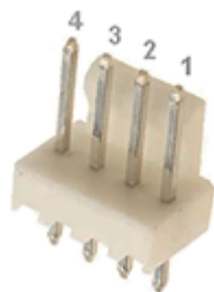
Pin 3,4: V+, Pin 1,2:-V-
