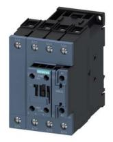
Contactor, AC-1, 110 A/400 V/40  $^{\circ}\text{C},$  S2, 4-pole, 175-280 V AC/DC, with varistor, 1 NO+1 NC, screw terminal
