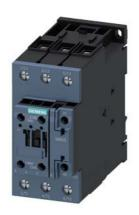
Power contactor, AC-3 80 A, 37 kW / 400 V 1 NO + 1 NC, 20-33 V AC/DC communication-capable, with varistor, 3-pole, size S2 screw terminals
