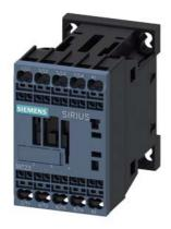
Contactor, AC-1, 22 A/400 V/40 °C, S00, 4-pole, 230 V AC, 50/60 Hz, Spring-type terminal
