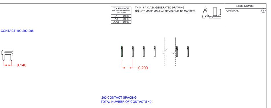
NOTE: CONTACTS ARE HELD IN A CARRIER FOR EASE OF ASSEMBLY
