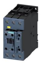
contactor, AC-3, 80 A/400 V/60  $^{\circ}\text{C}$  S2, 3-pole, 83-150 V AC/DC, F-PLC-IN, with varistor, 1 NC, screw terminal
