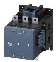
vacuum contactor, AC-3 500 A, 250 kW / 400 V AC (50-60 Hz) / DC operation 110-127 V AC/DC auxiliary contacts 2 NO + 2 NC 3-pole, frame size S12 busbar connections drive: conventional
