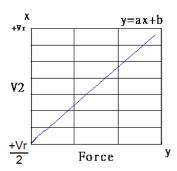
2. Using a fixed resistor R1 in a voltage divider configuration for an output V2 that increases with respect to added force.
