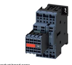
Power contactor, AC-3 25 A, 11 kW / 400 V 2 NO + 2 NC, 110 V AC, 50 Hz, 120 V, 60 Hz, 3-pole, Size S0, Spring type terminal Captive auxiliary switch
