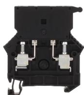
Fused terminal, Screw connection, Mounting type: Mounting rail TS 35/7.5 and TS 32, Rated cross-section: 10 mm<sup>2</sup>, Width: 8 mm, Colour: Black
