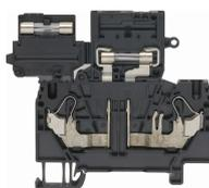
Fuse-disconnect terminal, Push-in connection, Mounting type: Mounting rail TS 35/7.5, Rated cross-section: 4 mm<sup>2</sup>, Width: 6 mm, Colour: Black
