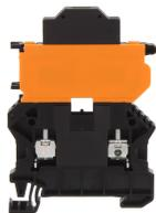
Fuse-disconnect terminal, Screw connection, Mounting type: Mounting rail TS 35/7.5, Rated cross-section: 4 mm<sup>2</sup>, Width: 6.1 mm, Colour: Black
