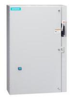
Non-reversing motor starter, Size 4, Three phase full voltage, Solid-state overload relay, OLR amp range 50-200A, Combination type, 200A fusible disconnect, 200A/600V fuse clip, Enclosure NEMA type 1, Indoor general purpose use, Standard width enclosure
