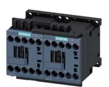
Reversing contactor assembly AC-3, 3 kW/400 V, 24 V DC 3-pole, Size S00 screw terminal electrical and mechanical interlock with integrated diode
