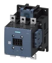
Traction contactor, AC-3 225 A, 110 kW / 400 V Coil 24 V DC x (0.7-1.25) PLC input 24-110 V DC Auxiliary contacts 2 NO + 2 NC 3-pole size S10 Busbar connections Coil connection: Spring-type terminal
