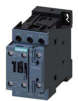
power contactor, AC-3 9 A, 4 kW / 400 V 1 NO + 1 NC, AC (50 / 60 Hz) DC operation 21-28 V AC/DC, 3-pole Size S0, screw terminal
