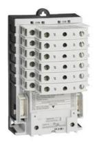
Electrically held lighting contactor, (convertible to mech. held), Amp rating 30A (tungsten 20A), 3 N.C. / 5 N.O. poles, 347V 60Hz coil, Noncombination type, Enclosure NEMA type (open), No enclosure
