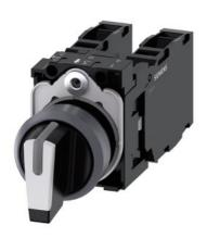
Selector switch, illuminable, 22 mm, round, plastic with metal front ring, white, selector switch, short, 3 switch positions I>O<II, momentary contact type, actuating angle 2x45°, 10:30h/12h/13:30h, with holder, 1 NO+1 NC, 1 NO+1 NC, screw terminal
