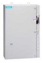
Non-reversing motor starter, Size 3, Three phase full voltage, Solid-state overload relay, OLR amp range 25-100A, 24VAC 50-60Hz coil, Combination type, 100A fusible disconnect, 100A/600V fuse clip, Enclosure NEMA type 4/12, Water/dust tight for outdoors, Standard width enclosure
