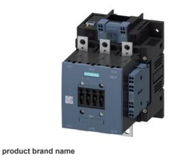
power contactor, AC-3 150 A, 75 kW / 400 V AC (50-60 Hz) / DC operation 21-27 AC/DC, 3 V auxiliary contacts 2 NO + 2 NC 3-pole, frame size S6 busbar connections drive: electronic with PLC interface 24 V DC spring-loaded terminal
