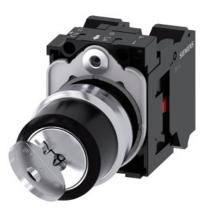
RONIS key-operated switch, 22 mm, round, metal, shiny, lock number SB30, with 2 keys, 2 switch positions O-I, latching, actuating angle 90°, 10:30h/13:30h, key removal O, with holder, 1 NC, 1 NC, spring-type terminal, possible special locks: SB31, 421, 455, upper case
