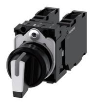
Selector switch, illuminable, 22 mm, round, plastic, white, selector switch, short, 3 switch positions I>O<II, momentary contact type, 10:30h/12h/13:30h, with holder, 2 x 1 NO+1 NC, screw terminal, with laser labeling, upper case and lower case, always upper case at beginning of line
