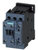
power contactor, AC-3 9 A, 4 kW / 400 V 1 NO + 1 NC, 220 V AC, 50 Hz 240 V, 60 Hz, 3-pole Size S0, screw terminal
