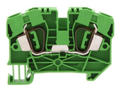
Feed-through terminal, Tension-spring connection, Mounting type: Mounting rail TS 35/7.5, Rated cross-section: 6 mm², Width: 8.1 mm, Colour: Green
