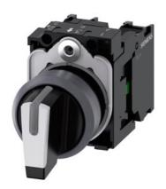
Selector switch, illuminable, 22 mm, round, plastic with metal front ring, white, selector switch, short, 3 switch positions I-O-II, latching, actuating angle  $2x45^\circ$ , 10:30h/12h/13:30h, with holder, 1 NO, 1 NO, screw terminal, with laser labeling, upper case
