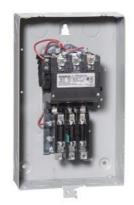
Non-reversing motor starter, Size 2 1/2, Three phase full voltage, Amb compensate bimetal OLrelay Contactor amp rating 60Amp 220 240/440 480VAC 60HZ coil, Non-combination type, Enclosure type 1, Indoor general purpose use
