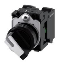
Selector switch, illuminable, 22 mm, round, plastic, white, selector switch, short, 2 switch positions O-I, latching, 10:30h/13:30h, with holder, 1 NO, 1 NC, spring-type terminal, with laser labeling, lower case
