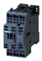
power contactor, AC-3 12 A, 5.5 kW / 400 V 1 NO + 1 NC, AC (50-60 Hz) DC operation 200-280 V AC/DC 3-pole, Size S0 Spring-type terminal
