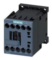
Coupling contactor relay, 4 NO, 24 V DC, 0.7  $\dots$  1.25\* US, Size S00, screw terminal suitable for PLC outputs
