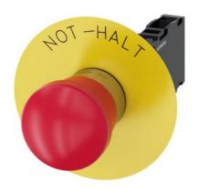
EMERGENCY STOP mushroom-type actuator, 22 mm, round, metal, shiny, red, 40 mm, positive latching, according to EN ISO 13850, pull-to-unlatch mechanism, with yellow backing plate, inscription: NOT-HALT, with holder, 1 NO+1 NC, screw terminal
