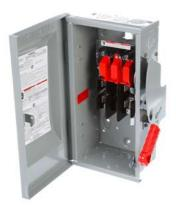
Siemens Low Voltage Circuit Protection Heavy Duty Safety Switch. 1-Pole 2-Wire and positive and negative ground Fused in a type 3R enclosure (outdoor). Rated 1000VDC (200A). Special features: photovoltaic rated, 10000 AIC disconnect.
