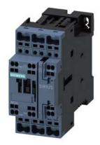
power contactor, AC-3 12 A, 5.5 kW / 400 V 1 NO + 1 NC, 24 V DC 3-pole, Size S0 Spring-type terminal
