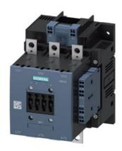
power contactor, AC-3 115 A, 55 kW / 400 V AC (50-60 Hz) / DC operation 220-240 V AC/DC auxiliary contacts 2 NO + 2 NC 3-pole, frame size S6 busbar connections drive: conventional spring-loaded terminal
