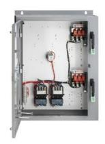
Duplex starter with alternator Size 0 Three phase full voltage Solid-state overload relay OLR amp range 5.5-22A 110VAC 50Hz / 120VAC 60Hz Coil Combination type Two 30A disconnect switches Enclosure NEMA type 4/12 Water/dust tight weather proof
