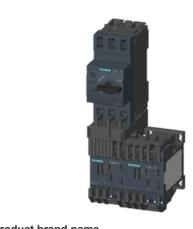
Load feeder fuseless, Reversing duty 400 V AC, Size S00 0.45...0.63 A 24 V DC Spring-type terminal for installation on standard mounting rail (also fulfills type of coordination 1) Type of coordination 2, Iq = 150 kA 1 NC (contactor)
