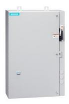
Non-reversing motor starter, Size 1, Three phase full voltage, Solid-state overload relay, OLR amp range 3-12A, 208VAC 60Hz coil, Combination type, 30A fusible disconnect, 30A/600V fuse clip, Enclosure NEMA type 4/12, Water/dust tight for outdoors, Extra-wide enclosure
