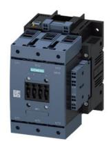
power contactor, AC-3 115 A, 55 kW / 400 V AC (50-60 Hz) / DC operation 21-27 AC/DC, 3 V auxiliary contacts 2 NO + 2 NC 3-pole, frame size S6 with box terminals drive: electronic with PLC interface 24 V DC spring-loaded terminal
