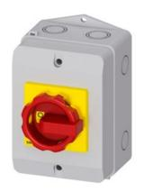
SENTRON, Switch disconnector 3LD, emergency switching-off switch, 3-pole, Iu: 32 A, operating power / at AC-23 A 400 V: 11.5 kW, molded-plastic encapsulation for inch cable gland, rotary operating mechanism, red/yellow
