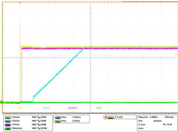
Figure 20. Startup via input voltage (No load)
