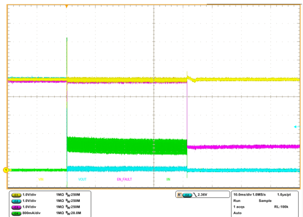
Figure 29. Output short-circuit during operation
