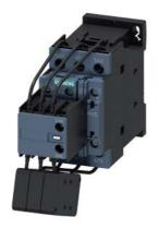
Capacitor contactor, AC-6b 16.7 kVAr, / 400 V 1 NO + 2 NC, 220 V AC, 50 Hz 240 V, 60 Hz 3-pole, Size S0 screw terminal
