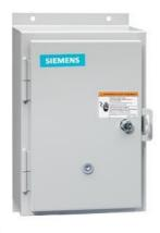
Non-reversing motor starter, Size 1 3/4, Three phase full voltage, Solidstate overload relay, OLR amp range 10-40A, 208VAC 60Hz coil, Noncombination type, Enclosure type 12, Dust/drip proof for indoors, Extrawide enclosure
