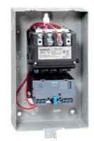
Non-reversing motor starter Size 00 Three phase full voltage Solid-state overload relay OLRelay amp range 3-12A 190-220/220-240V 50/60HZ coil Combination type Indoor general purpose use
