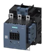
power contactor, AC-3 150 A, 75 kW / 400 V AC (50-60 Hz) / DC operation 440-480 V AC/DC auxiliary contacts 2 NO + 2 NC 3-pole, frame size S6 busbar connections drive: conventional spring-loaded terminal
