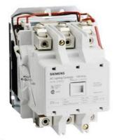
Mechanically held lighting contactor, Contactor amp rating 100A, 0 N.C. / 2 N.O. poles, 220VAC 50HZ/240VAC 60HZ coil, Non-combination type, Enclosure NEMA type (open), No enclosure
