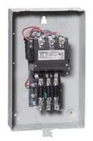
Non-reversing motor starter, Size 2 1/2, Single phase, 2-pole, Amb compensate bimetal OLrelay Contactor amp rating 60Amp 110 120/220 240VAC 60HZ coil, Non-combination type, Enclosure type 1, Indoor general purpose use
