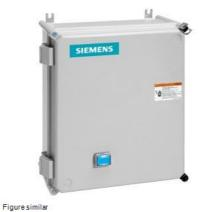
Non-reversing motor starter, Size 1, Three phase full voltage, Solid-state overload relay, OLR amp range 0.25-1A, Non-combination type, Enclosure type 4X fiberglass, Water/dust tight noncorrosive, Standard width enclosure
