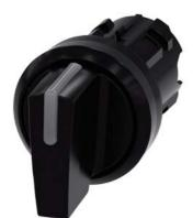
Illuminable selector switch, 22 mm, round, plastic, black, Selector switch short, 3 switch positions I>O<II, momentary contact type, actuating angle  $2x45^{\circ}$ , 10:30h/12h/13:30h
