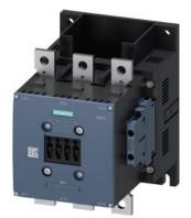
Contactor, AC-1, 400 A/690 V/40  $^\circ\text{C},$  S10, 3-pole, without operating mechanism, 2NO+2NC, connection bar/ screw terminal
