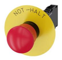
EMERGENCY STOP mushroom-type actuator, 22 mm, round, plastic, red, 40 mm, positive latching, according to EN ISO 13850, rotate-to-unlatch, with yellow backing plate, inscription: NOT-HALT, with holder, 1 NO+1 NC, screw terminal, Z=20-unit packaging
