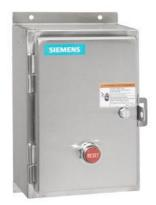
Reversing motor starter, Size 3 1/2, Three phase full voltage, Amb. compensate bimetal OLR, Contactor amp rating 115A, Non-combination type, Encl. type 4X 304 S. Steel, Water/dust tight noncorrosive
