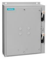
Duplex starter w/ alternator, Size 1, Three phase full voltage, Amb. compensate bimetal OLR, contactor A rating 27A, 110V 50Hz / 120V 60Hz coil, Combination type, Two 25A circuit breakers, Enclosure NEMA type 12, Dust/drip proof for indoors
